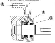
1 Fitting for hose with inside diameter 10mm
